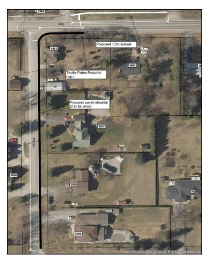
Figure 1: Conceptual drawing of pedestrian facility improvements in Solina.
