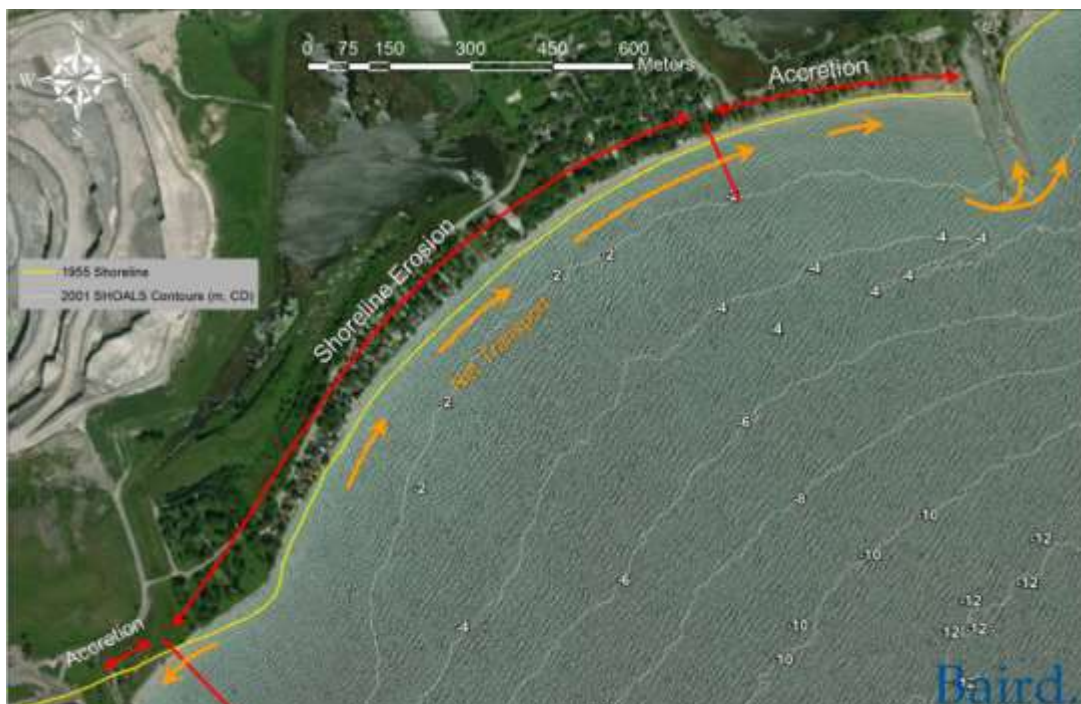
Figure 0.1: Comparison of 1955 and 2014 shorelines showing erosion and accretion areas, and net direction of longshore sediment transport
