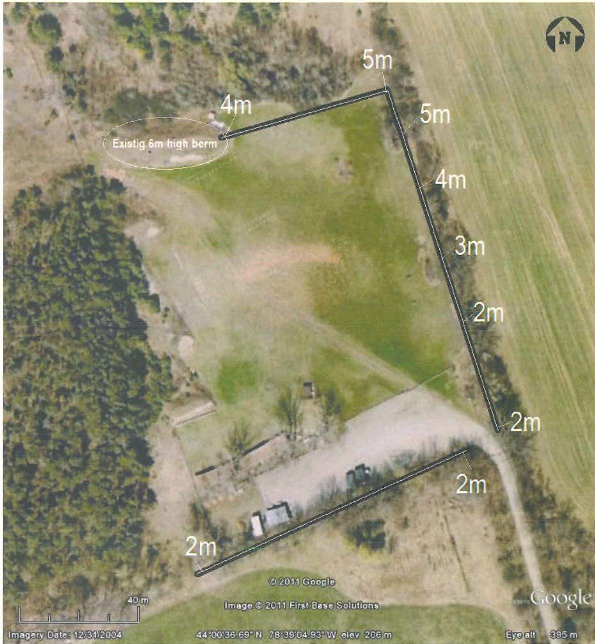
Figure 6: Barrier Heights and Locations
