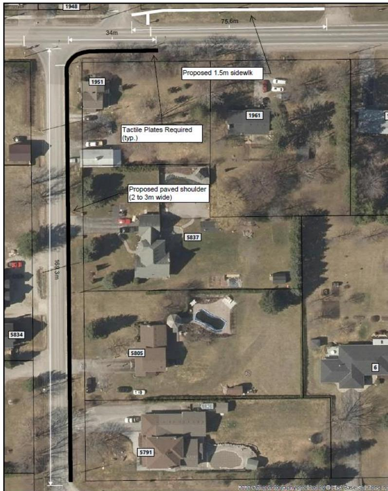
Figure 1: Conceptual drawing of pedestrian facility improvements in Solina.
